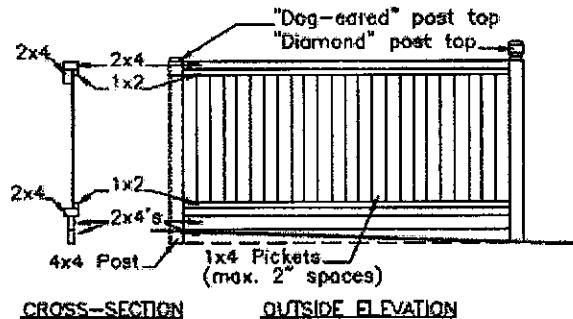
CROSS-SECTION      OUTSIDE ELEVATION
